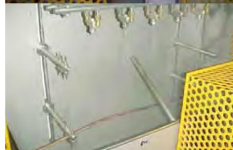
MICO® cable during mechanical test (950°C again for 15 minutes then mechanical impact directly on the cable)
