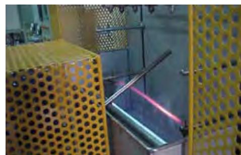
MICO® cable during water test (650°C for 15 minutes, then water crush trough sprinklers)
