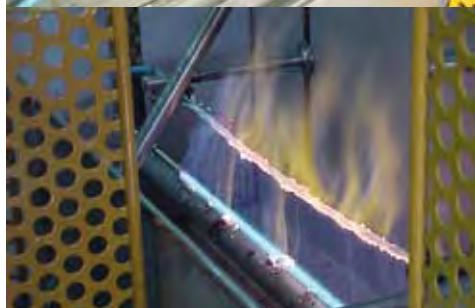
Standard cable failure after few minutes of fire test
